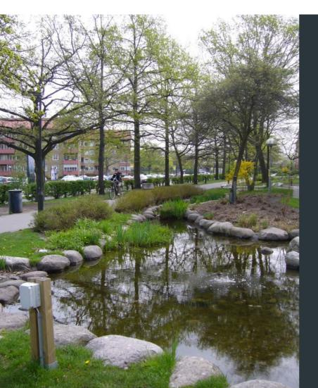
Sustainable drainage systems can be designed to provide attractive green and blue spaces for people, as well as preventing flooding, improving water quality and supporting biodiversity. Photo: SUSDRAIN
